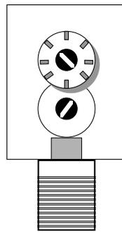
**Pressure Switch** - The pressure switch senses a drop in pressure and activates a device or relay. They are available in both single point actuation and differential pressure. This mode of control relies primarily on the pump curve characteristics as they relate to pressure output. (Indirect Measurement of Flow)
