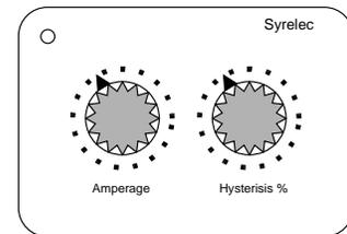
**Current Sensing Relay** - The relay monitors amperage draw created by the motor as the flow increases through the pump. This amperage is set to a specific "on" time based on engineer requested sequencing. It is an indirect measurement of flow, but highly accurate. (Indirect Measurement of Flow via amperage)
