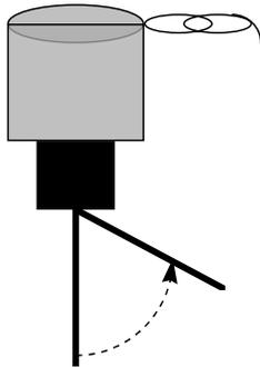
**Flow Switch** - senses water flow against a paddle which is in the water stream. Paddle moves a "cam" within the body which actuates next sequence. This is an accurate means of measuring flow, however, can be subject to corrosion and obstruction. (Direct Measurement of Flow)
