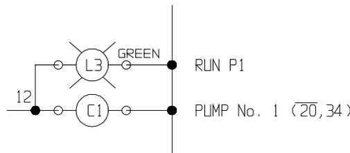
**Pump run indicator and contact coil in parallel. The coil closes contacts starting a motor.**
