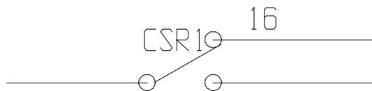
**Current sensing relay switch closes actuating a control relay to start or shut down a motor.**
