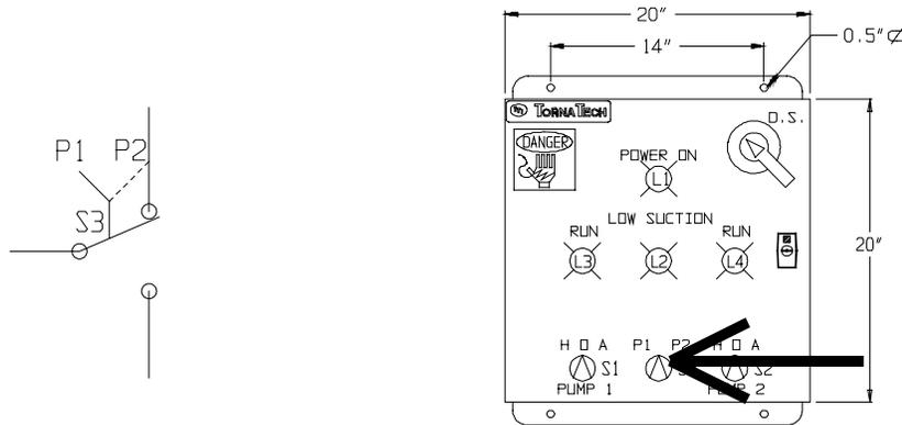
*Manual alternator switch determines which pump leads.*
