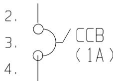
**The control circuit breaker prevents current overloads in the controls' sensitive components.**
