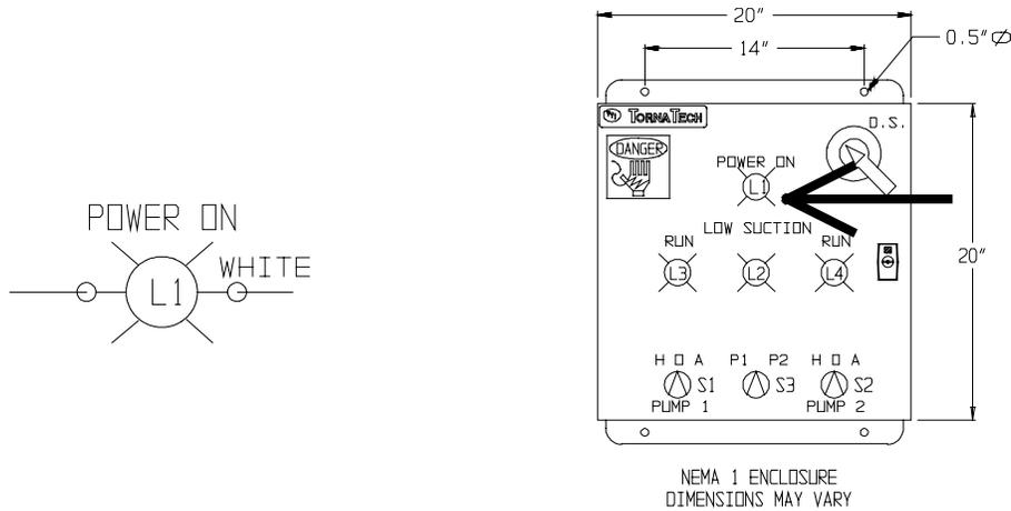
**The Power On pilot light informs the controls operator that the panel is live.**
