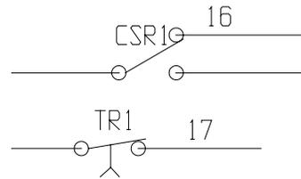
***Timing Relay holds the contact for a set period of time in order to prevent pump cycling.***
