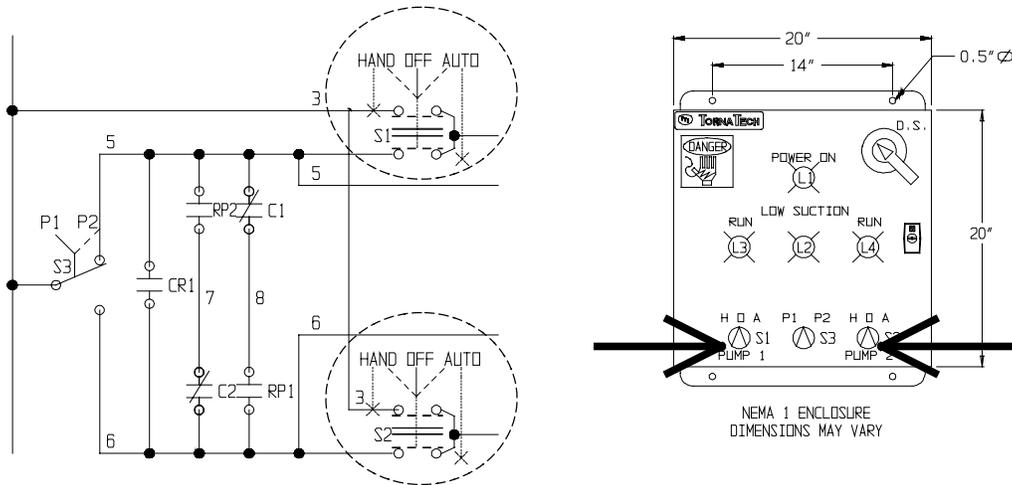
**Pump Shunting Circuit holds key to pump sequencing. The circuit is only activated when the pumps are placed in the AUTO position.**
