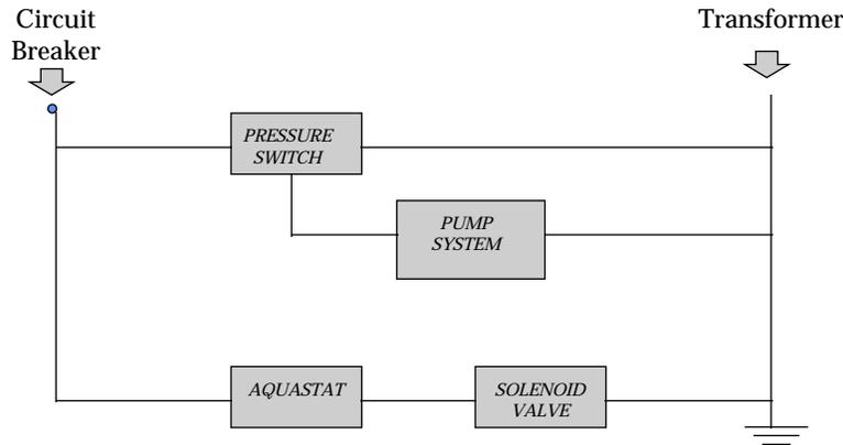
*Block Diagram of Pump Protection Circuit*
