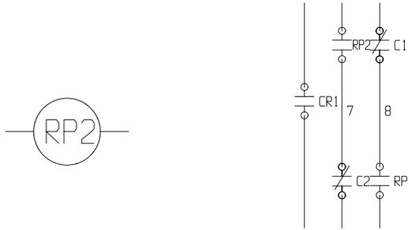
**Control Relay Coil actuates the motor starter contacts inside the shunting circuit.**
