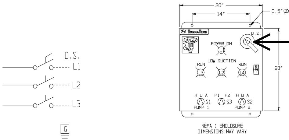
*Schematic of Disconnect Switch. The location of the switch on the panel is indicated by the arrow.*
