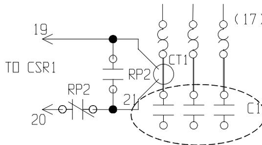
**Contacts (RP2) close to start the motor running or open to shut one down.
