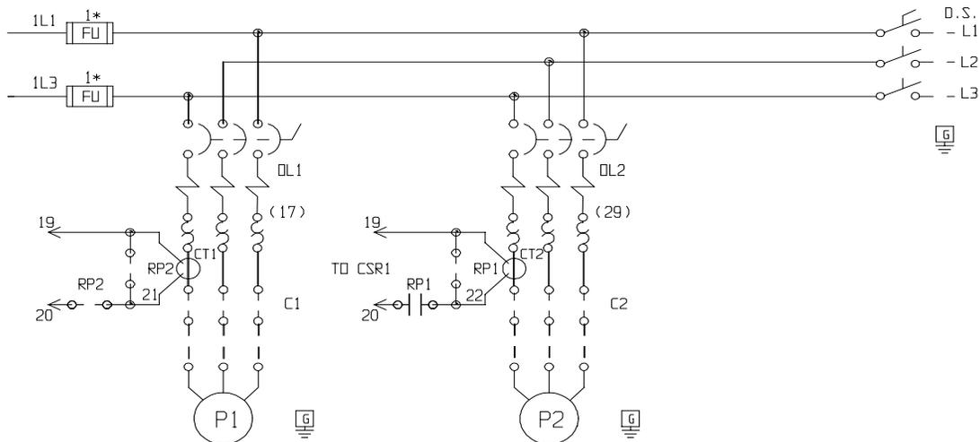
**Main Disconnect and Motor Protection Circuit. Note that the lower segment of the diagram (marked “P1” and “P2”) represents the motors and their respective starters.**
