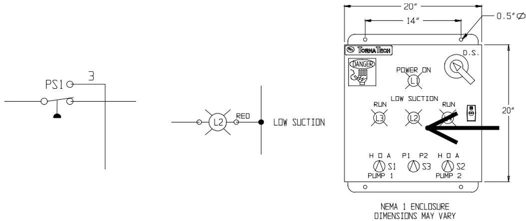
**Fig.# 21: Low suction pressure switch shuts down system and warns by lighting pilot.**
