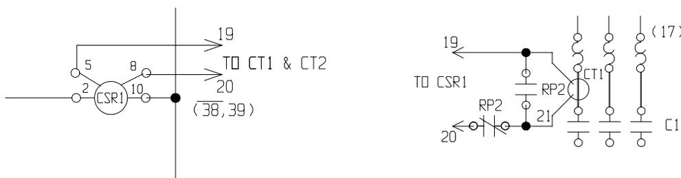
**Current Sensing Relay.** In combination with a control relay, the CSR activates a current transformer in the starter (part of the contact arrangement) to start the motor. The numbers 19 and 20 marking the arrows indicate a connection to the matching numbers on the motor lead.
