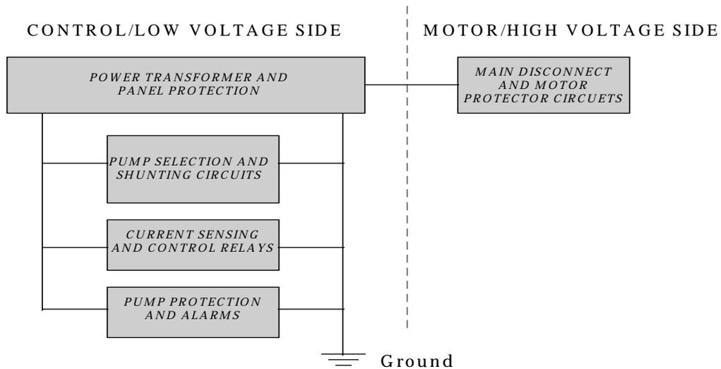
**Block Diagram of Complete Control Circuit**
