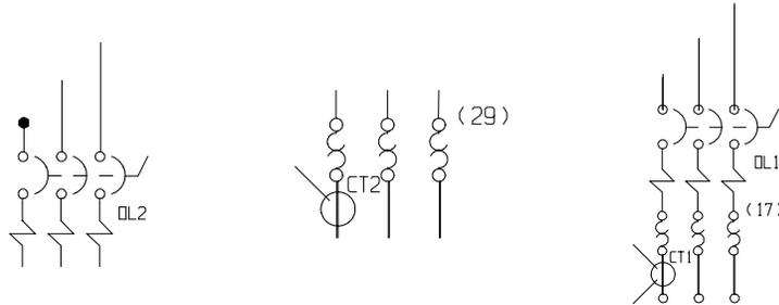
**The short circuit protector (left) and overload protector (middle) combine to form a complete motor protector circuit (right).** Within the controller, these components are integrated into a single component called an overload relay. The device has a setting for the maximum allowable amperage, and a two push button circuit breaker (pushing in the red button opens the circuit / pushing in the white button closes the circuit).
