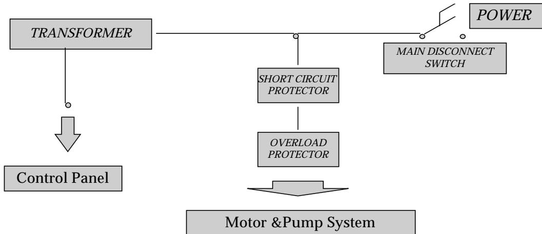
*Block Diagram of Main Disconnect and Motor Protector Circuits*
