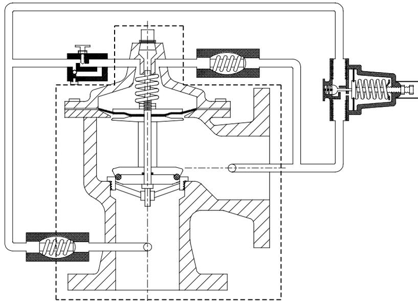
*The dashed line separates the internal main body valve and the external pilot assembly.*
