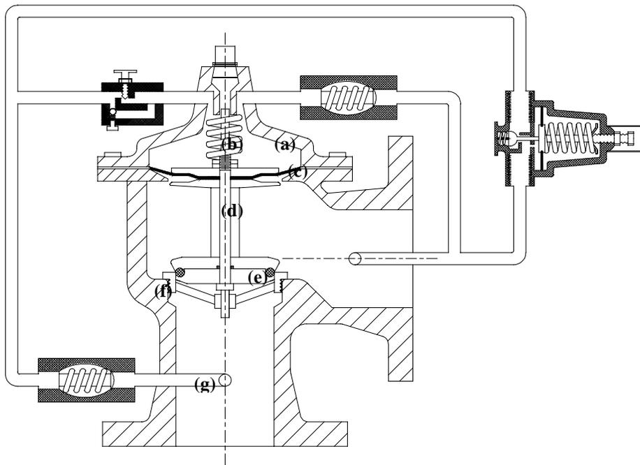
***Main body valve components and subassemblies.***
