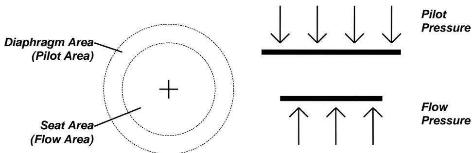
**Fig.# 5: The pilot pressure “wins out” over the flow pressure due to hydraulic leverage advantage.**
