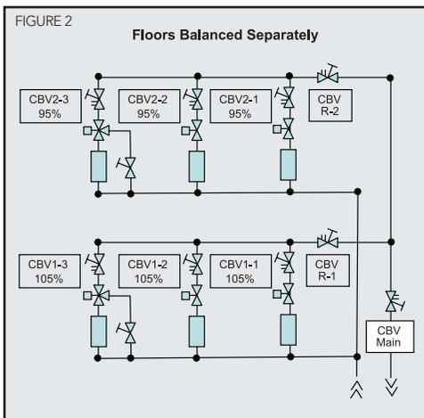
there is interaction between valves, and as any one is throttled, the flow through the others increases. Experienced balancers can often predict the amount of compensation required for this interaction and can adjust all valves to achieve a common flow through all in just one pass.
