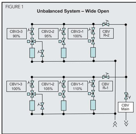
**5** To balance the floors together, leave the riser balancing valve of the most disadvantaged floor wide open (Figure 3, CBV R-2). Adjust the riser valves of other floors, until all floors are at an equal flowrate.
